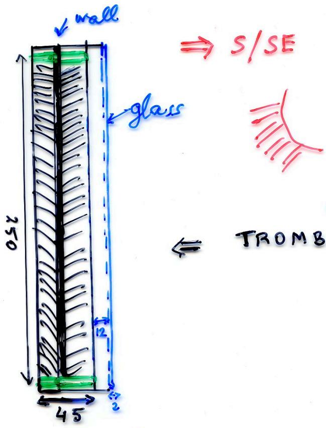
**WINTER:** During day, solar chimney behind glasses heats the room by convection through the holes. During night, heating thanks to the 12 hours phase-shift, (and  $2 \times 6$  h. phase shift on all other walls)
