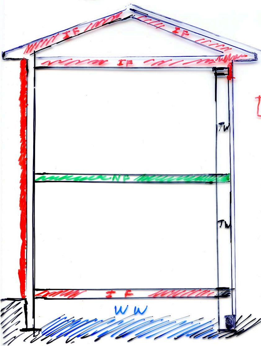
**SUMMER:** Cooling thanks to the humid basement (sea water level is only 30 cm below WW, and good transfer of humidity).
