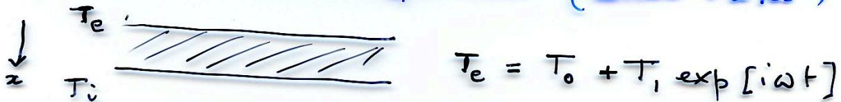
$$\Rightarrow T(t, x) = T_0 + T_1 \exp[-x/l] \exp[i(\omega t - x/l)]$$
