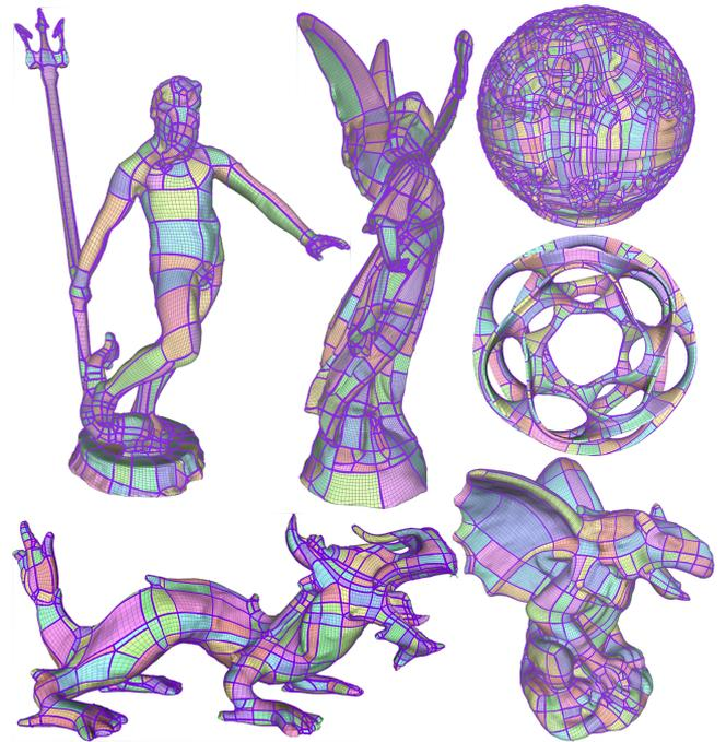
**Figure 6:** Complex meshes requiring a few t-junctions.
